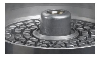
The intricately channeled base provides a large footprint to fully support the element under pressure, ensuring uniform loading of the element. Ultra-clean oil flows through the channels into the clean oil stream.
